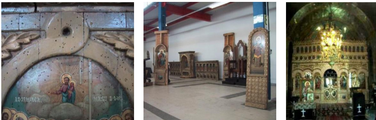
FIG. 1. The first iconostasis treated with gamma rays at IRASM, in 2002 [1]: detail of the decay attack; dismantled, in the IRASM warehouse; in the church, after complete restoration.
