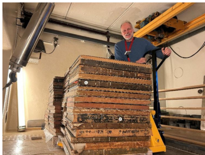
FIG. 3. ©ARC-Nucléart Installation of archives in the irradiation chamber for fungicidal treatment.
