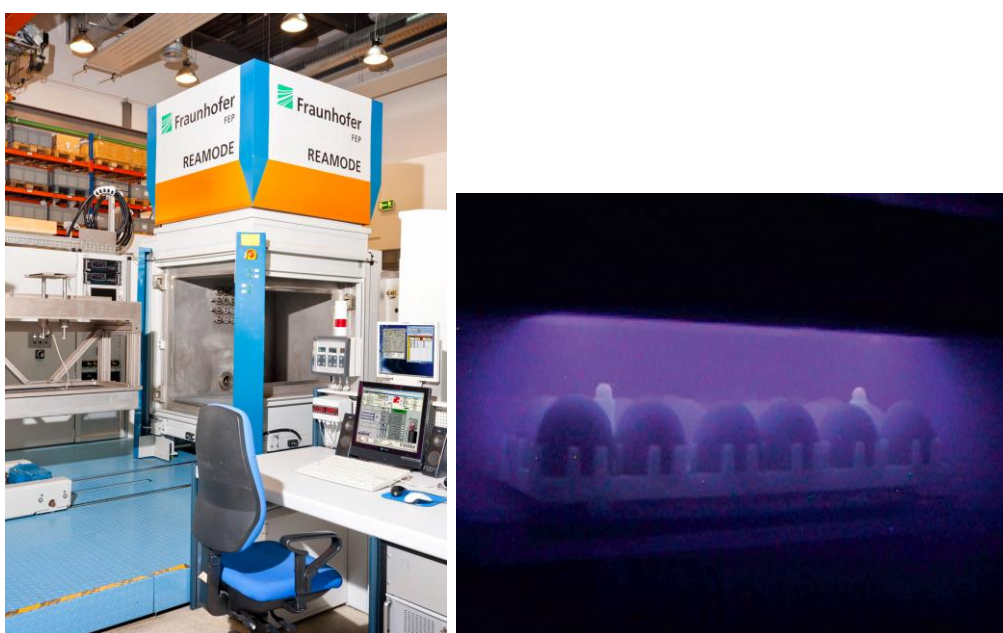
The REAMODE facility at the Fraunhofer FEP Laboratory, Dresden, for the experimental study of modifying organic material (left) and eggs under the electron beam for disinfection (right).
