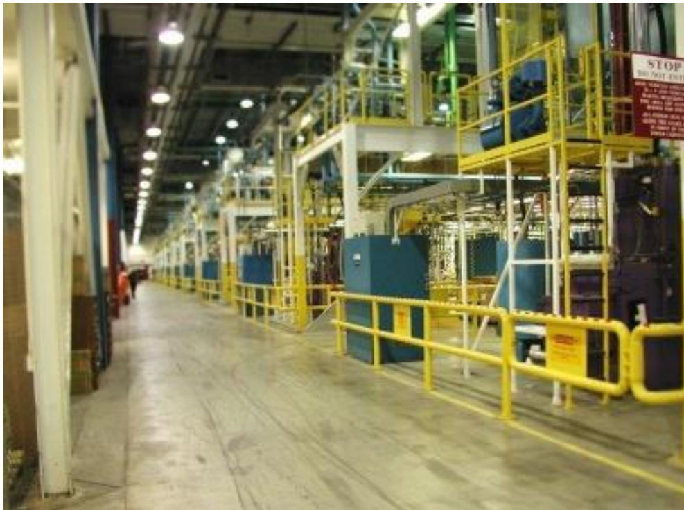
Industrial in-line aluminium surface treatment with e-beam.
