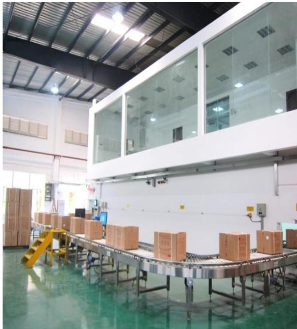
The layout of the conveyor must be such that the area where non-sterile products are loaded and the area where sterile products are unloaded are physically segregated. Loading and unloading at dedicated stations can be manual or it can be automated, for example to unstack and restack pallets.
