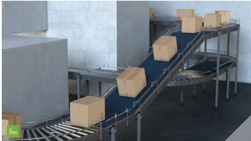
Product handling can be supplied by the accelerator manufacturer or by other specialized companies. When the accelerator and the product handling are not provided by the same supplier, the integration must be carefully planned.
