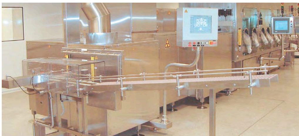
Figure 108. STERSTAR™ System for In-line EB Surface Decontamination
