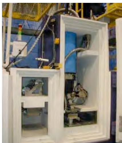
Figure 76. Self-shielded 500 keV Electron Beam for Shrinkable Film
