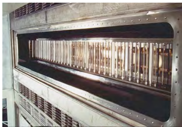
Figure 32. Segmented Low-energy EB Filament Array without Beam Window
