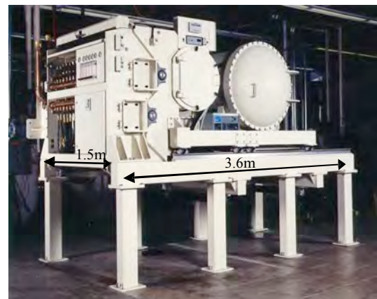
Figure 31. Low-energy EB unit
