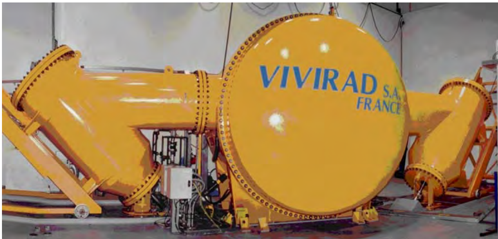
Figure 29. Vivirad 2 MeV with Two Cross-firing Beams from One Power Supply
