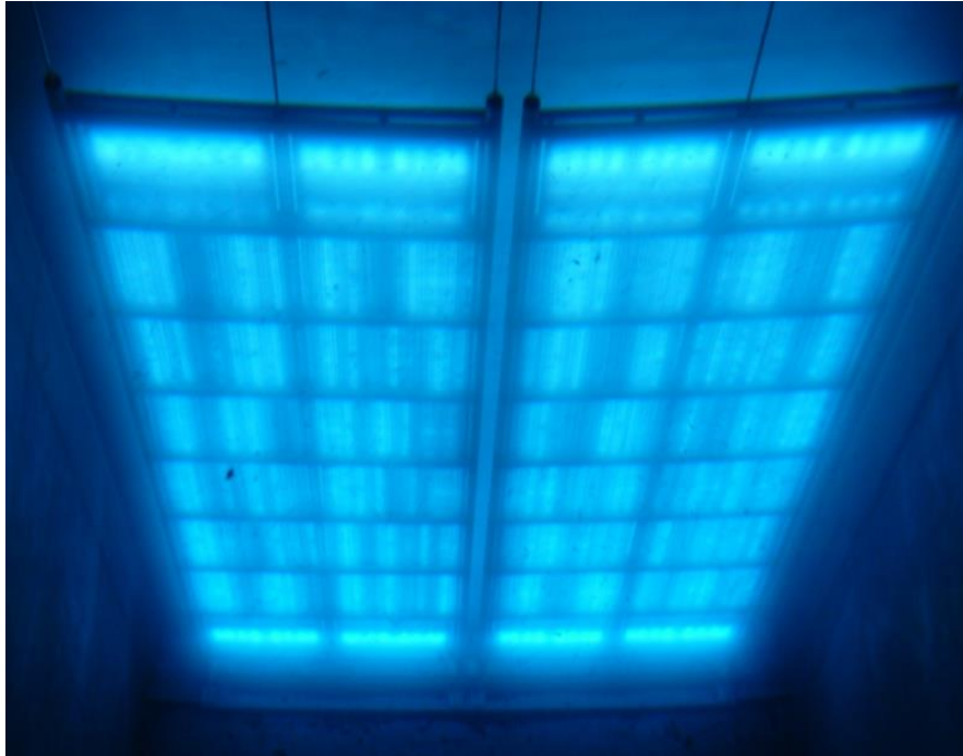
Figure 2: A source rack loaded with multiple cobalt-60 sources within the storage pool of a radiation processing facility. Illustration courtesy of STERIS AST.
