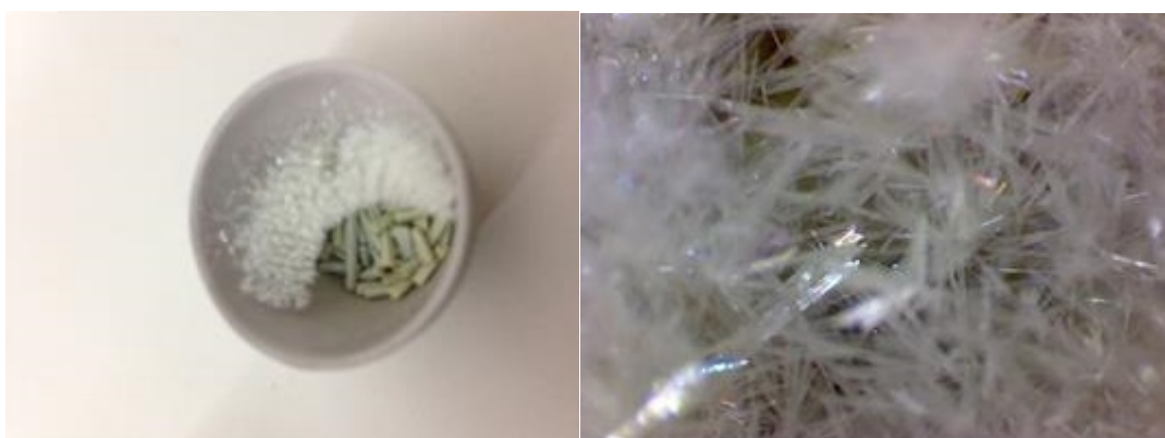
FIGURE 1 – RADIATION-THERMAL TREATMENT PROCESSING ON SPENT HCC CATALYST FROM UPPER ZONE: ALUMINA CRUCIBLE AND CRYSTAL FORMED AFTER ELECTRON BEAM IRRADIATION.
