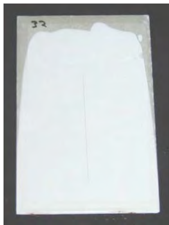
Figure 86. EB Coating after 1000 Hours Salt Spray
