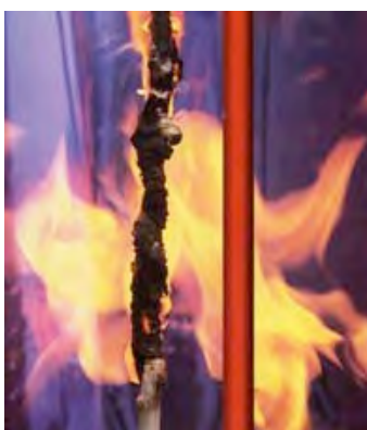
Figure 72. EB Crosslinked Flame Retardant Insulation
