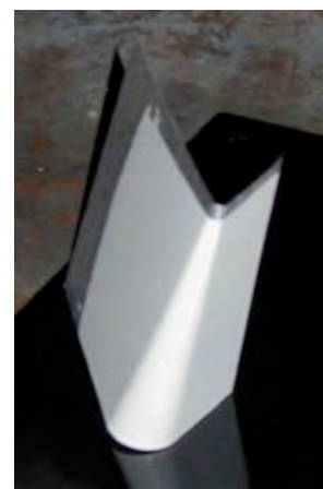
Figure 87. EB Coating after Mandrel Bend Test
