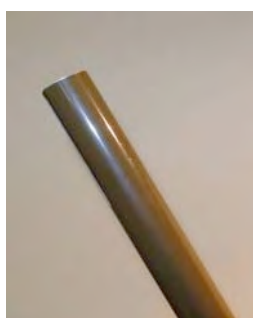
Figure 88. EB Cured Coating on Tubular Aluminum
